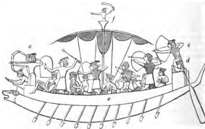
Ancient Egyptian War-galley; the sail being clewed up during the action. (Thebes.) a, raised forecabin, in which the archers were posted; c, another post for the archers, and the pilot, d; e, a bulwark, to protect the rowers; f, slingers, in the top.
